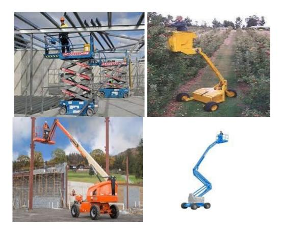
Figure 6 – Examples of mobile elevated Work platforms and the great variety of sizes and uses. The top two EWP's only extend to a working height of five metres and weigh less than one tonne. The bottom two EWP's extend to a working height over 11 metres and weight over five tonnes.
