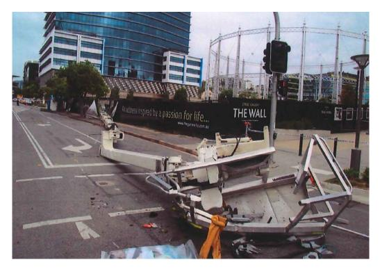
Figure 4 - Final position of the EWP basket on Longland Street. The front of the basket has been cut away by emergency services.
