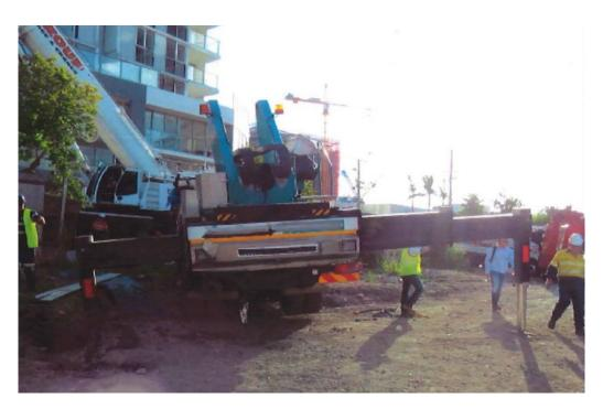
Figure 5 – The subject EWP after being recovered and "uprighted" but not returned to its original position. Note the rear outrigger "arm" on the passenger's side is not fully deployed to 3 metres unlike the driver's side leg. It was half deployed at 1.4 metres which reduced the "spread" of the load.
