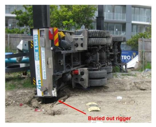
Figure 6 – Note the EWP in situ before being "uprighted" and buried passenger's side outrigger leg. The hard gravel crust can be seen but not the soft clay underneath.
