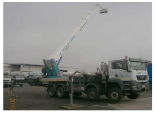
Figure 2 - Example of a similar Wumag-Palfinger WT 700 EWP in operation: note only the front outrigger legs and pads and crew bucket on this vehicle
