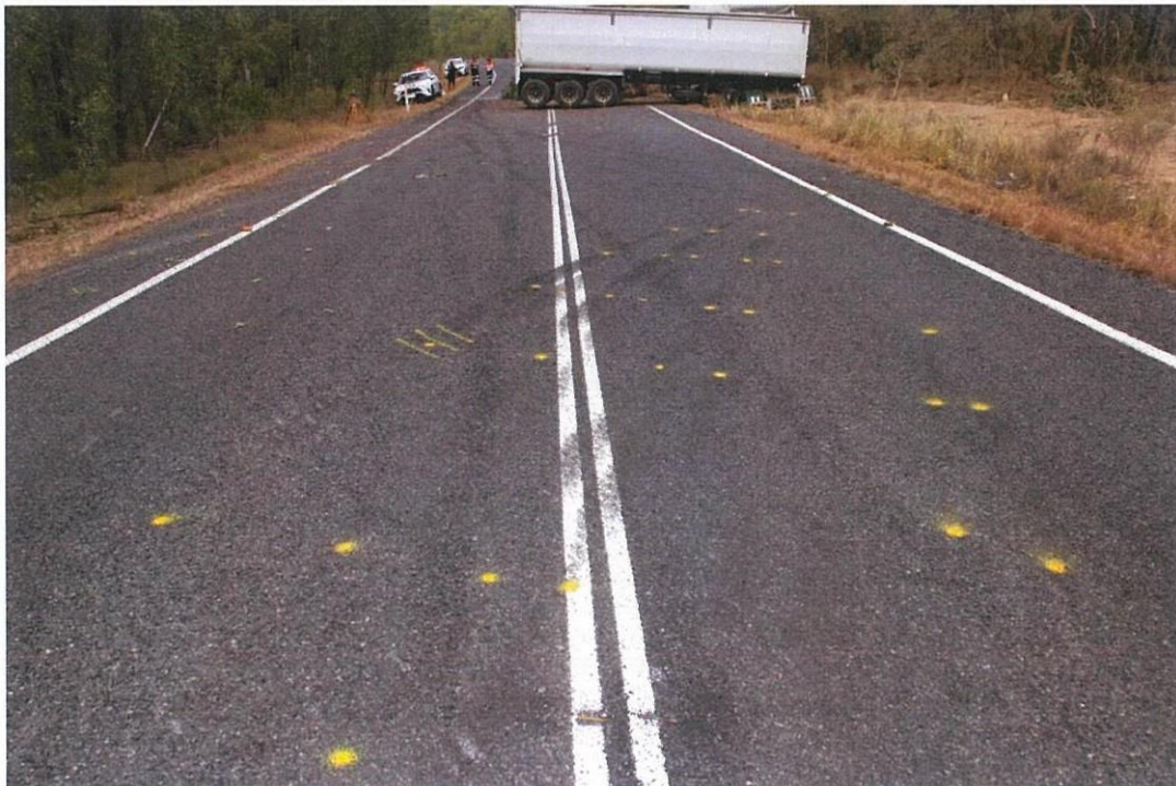
Wheel tracks crossing bitumen east to west close up. Right to left – PM, Trailer A, Trailer B.
