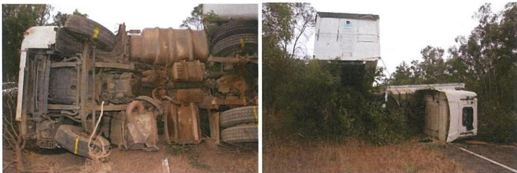
Image showing scrapes and damaged undercarriage of PM from contact & Image showing A Trailer free of coupling resting on rear left of PM.
