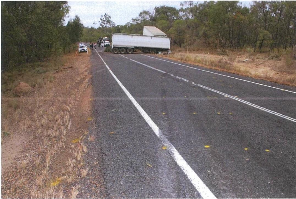
Wheel tracks re-entering bitumen close up. Right to left – Trailer A, Trailer B.
