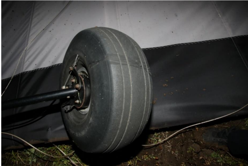
Image 14: Right front wheel showing impact marks of power lines.
