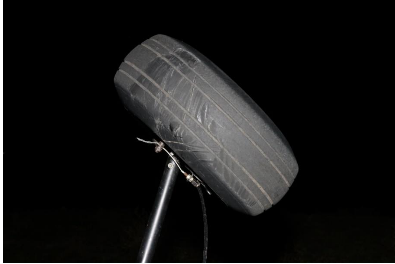
Image 13: Left front wheel showing impact marks of power lines.
